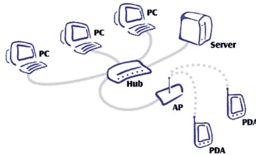
Figure 2 – LAN Extended with WLAN
