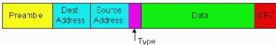
Figure 5 – Structure of an Ethernet Frame
